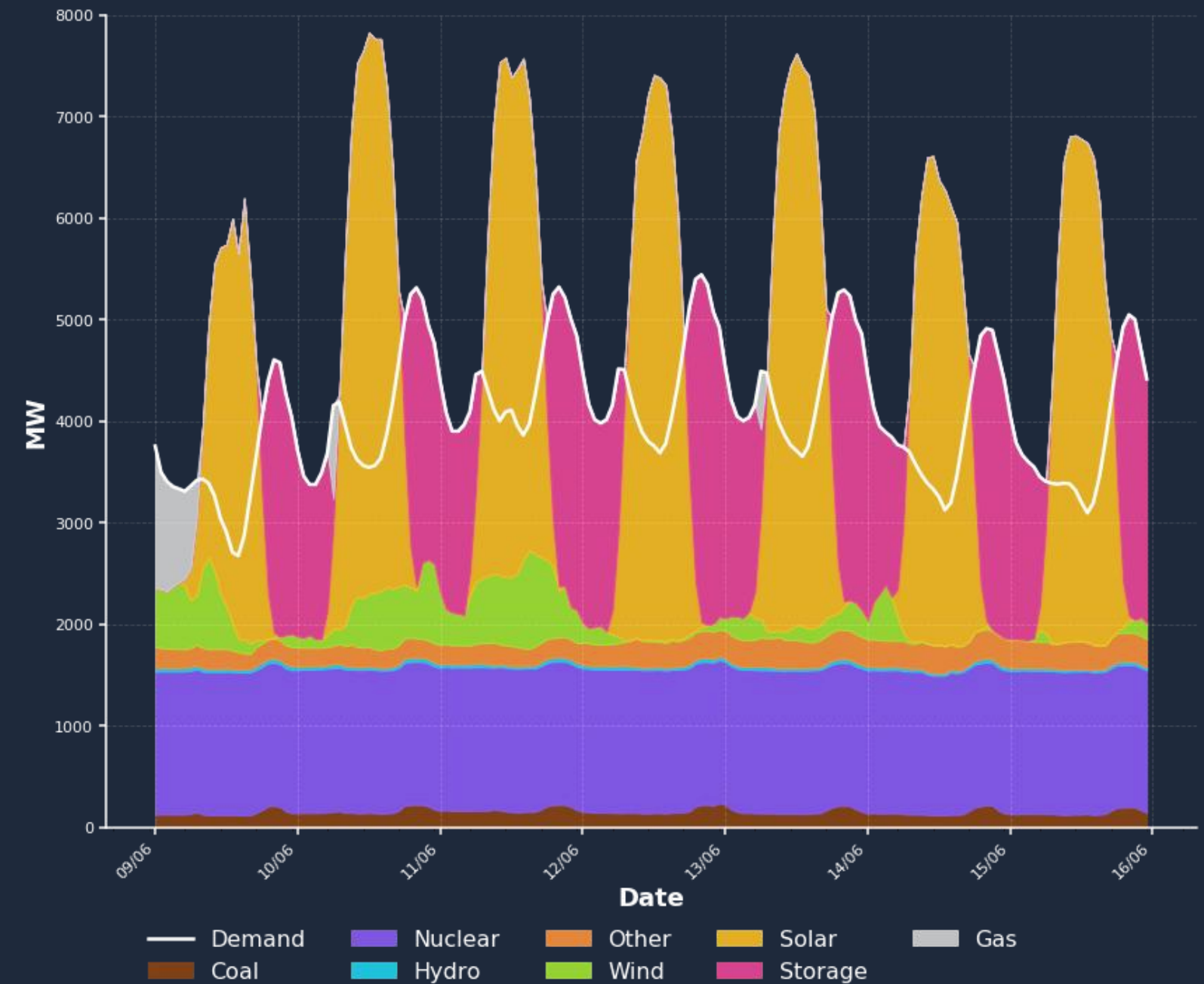
Figure 16. Storage has the potential to fill in demand and supply gaps with excess solar power
